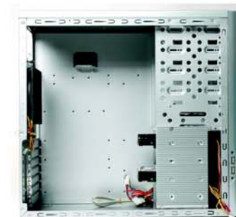
5. Mount the HDD as shown in the figure. (You must attach a pad for preventing heat conduction and vibration on each edge of the HDD before mounting the HDD in the bay.)
