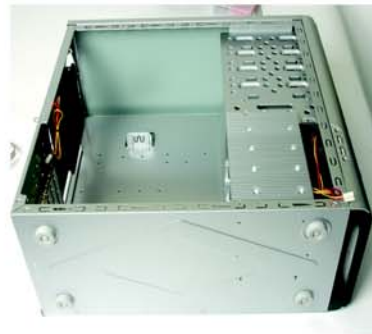
2. Before you mount a HDD in the 3.5" bay, you must lay down the main body first as shown in the figure.
