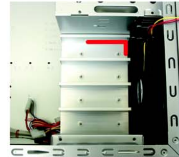
4. Align the HDD with the marked area in the figure and mount it there.
